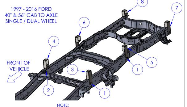
5/8" HOLES MUST BE DRILLED IN FRAME TO MOUNT FRONT AND CENTER LEVEL LOKS. REAR LEVEL LOKS WILL MOUNT IN EXISTING HOLES IN FRAME. IF NECESSARY, RE-DRILL THESE HOLES TO 5/8".
